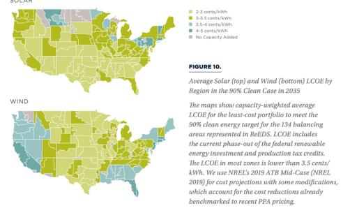
Source: 2035 Report: Plummeting Solar, Wind, and Battery Costs Can Accelerate our Clean Electricity Future. (June 2020).
